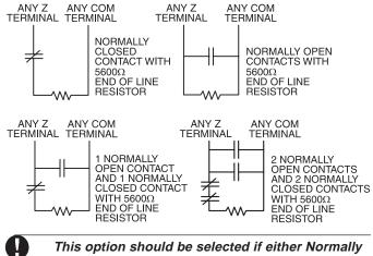
This option should be selected if either Norma Closed (NC) or Normally Open (NO) detection devices or contacts are being used.
