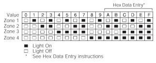
Press any of the Emergency Keys (Fire, Auxiliary or Panic) to advance to the next digit. When all the digits in a section have been viewed, the panel will exit the section; the Ready Light will turn OFF and the Armed light will turn ON, waiting for the next three-digit programming section number to be entered. Press the [#] key to exit the section
